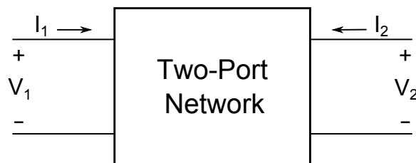
Fig. 2.2. A schematic representation of a two-port network.
